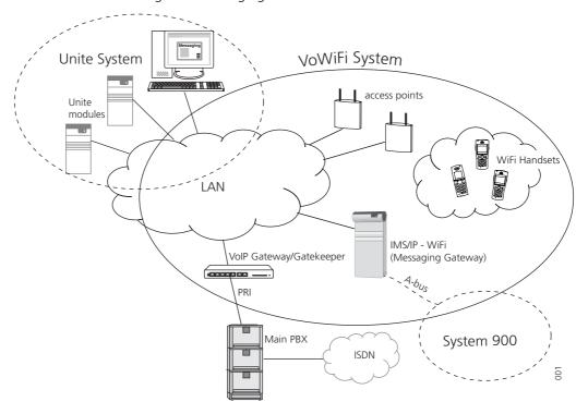
Figure 1. IMS/IP-WiFi connected to the LAN
